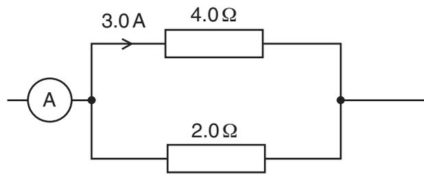
The current in the  $4.0\ \Omega$  resistor is  $3.0\ \text{A}$ .
